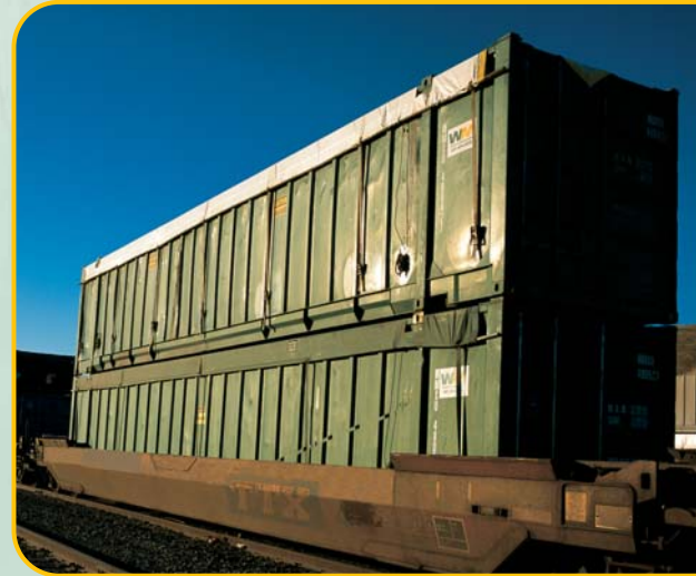
Intermodal rail containers allow solid wastes to be transported by truck and by rail to Waste Management landfills throughout North America.
